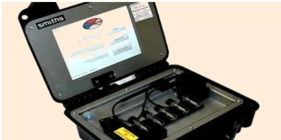
RespondIR verifies the identity of an unknown solid or liquid
